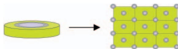
Figure 6. Schematic representation of dendrimer supermolecule as a disk and of the model for the rectangular columnar mesophase [green: fluorophilic layer F(CF 2 ) 8 ; grey: lipophilic layer (CH 2 ) 2 ; blue: hydrophilic layer (dendrimer-NH 3 + OOC)].
